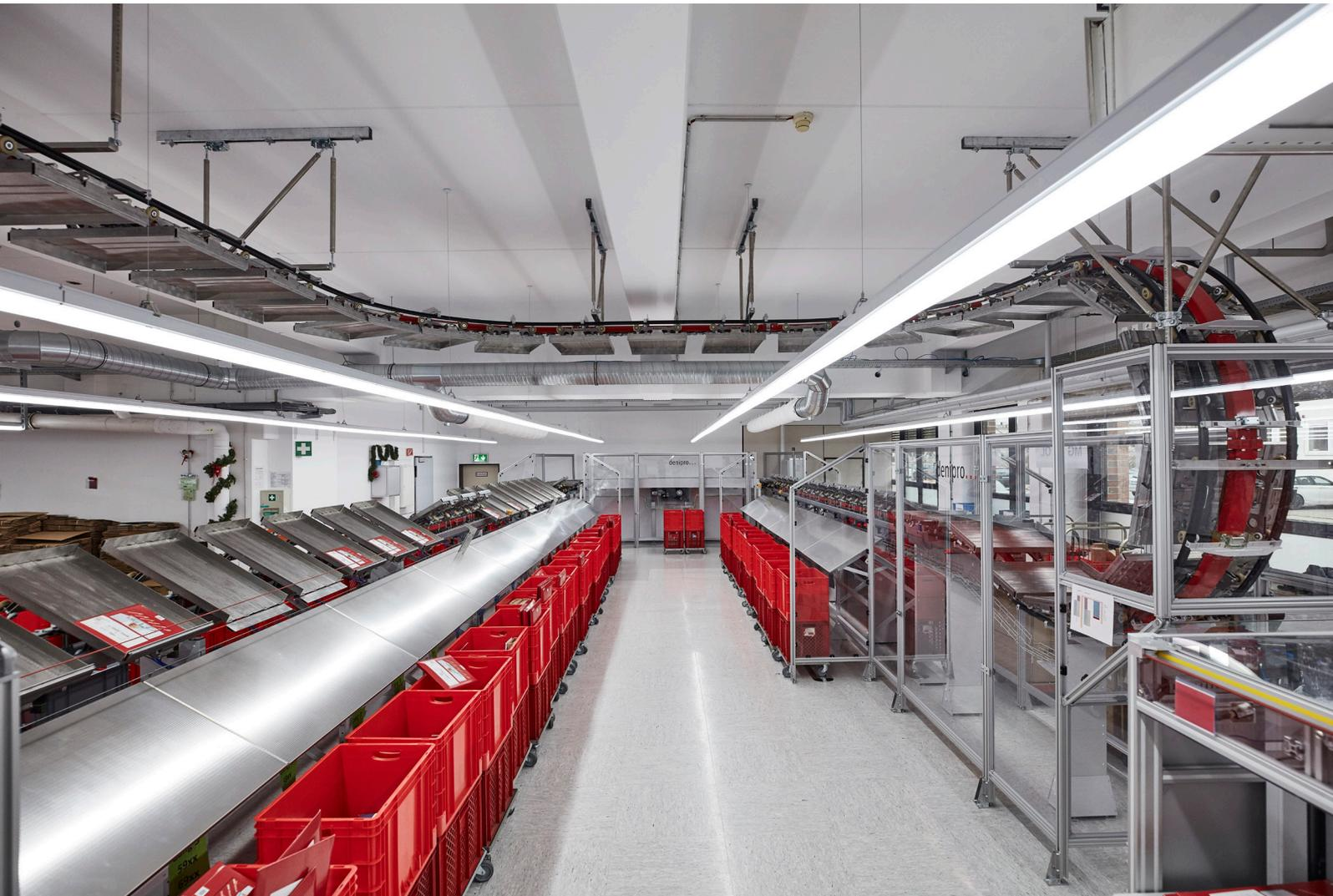
Denisort is an innovative tilt-tray sorter that combines conveying, order picking and sorting in one seamless and scalable system with universal applications across a wide range of intra-logistic processes. The basis is a carrier chain that runs energy-efficiently and quietly on low-friction rollers in a steel profile. The system thus enables individual solutions with a completely free layout in all dimensions, even across several levels.
