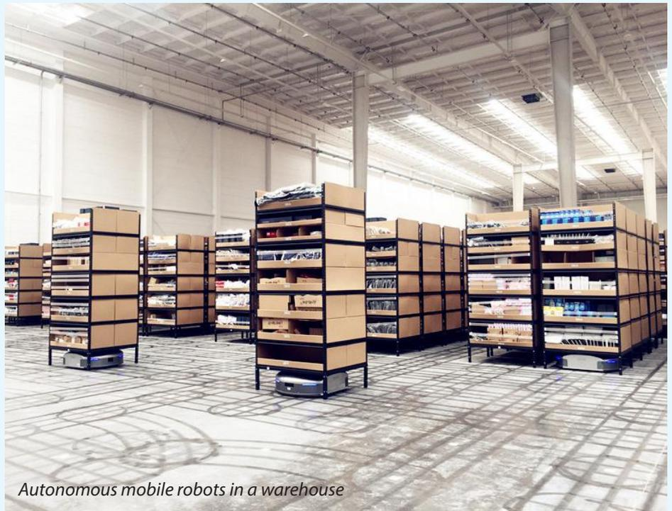
*Autonomous mobile robots in a warehouse*
